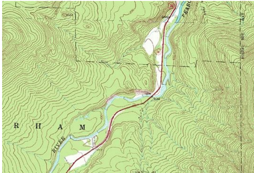
Figure 1 Topography suitable to dam construction. Steep slopes on both sides of the river will allow for a confined storage basin and a dam of reasonable length.
